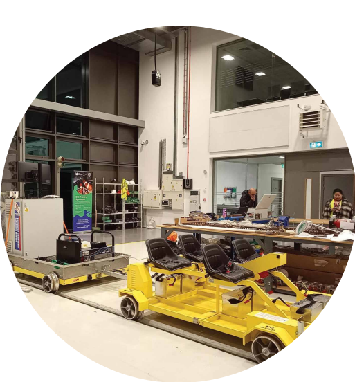
Preliminary testing of a mobile stabilisation platform setup at the National College for Advanced Transport & Infrastructure in Birmingham, UK. The platform (rear), control unit (centre) and drive cart (front) were investigated for vibrational characteristics along a section of railway in preparation for the deployment of quantum sensors.
